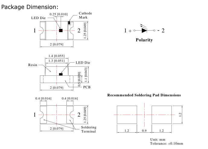
1. Soldering terminal may shift in x, y direction.
